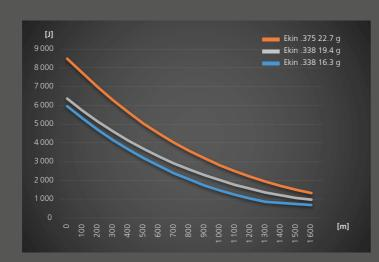
.375 SWISS P Ball delivers a better ballistic coefficient than the .338 LM HPBT Match bullets. In other words, the bullet loses less speed and therefore achieves a higher target energy, simultaneously extending the operational distance within the supersonic range.
